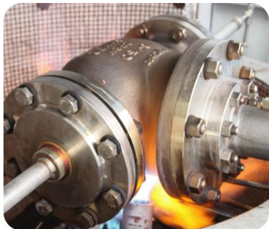
Fire safety testing on an 6 in. Top Entry Ball Valve
