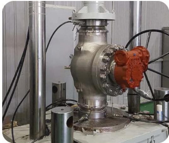
Hydraulic testing on an 10 in. Top Entry Ball Valve
